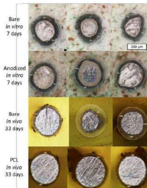
Figure 1. Representative transverse cross-sections of bare and coated wires after degradation in the indicated environment and duration.
