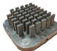
Fig. 1. Additively manufactured samples still attached to the building platform.
